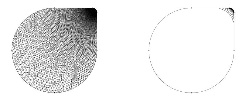
5484 internal nodes, 3829 C.G. iterates, 9243 gradient steps, divergence ranges from 1.18 to 12.7
